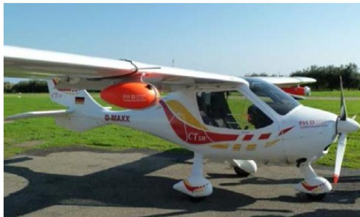
Figure 3.2: Flight Design CT deployed by the University of Applied Sciences of Düsseldorf for fast response volcanic cloud measurements
