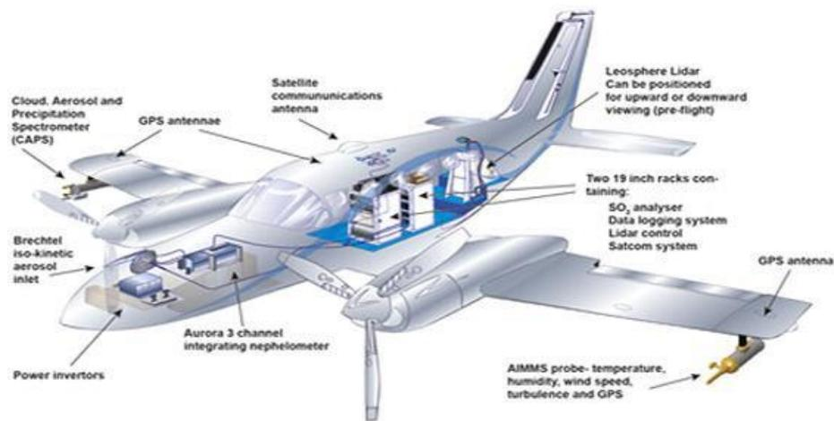
Figure 3.1: UK Met Office Civil Contingency Aircraft for fast response measurements of volcanic ash clouds including lidar remote sensing measurements (MOCCA)
